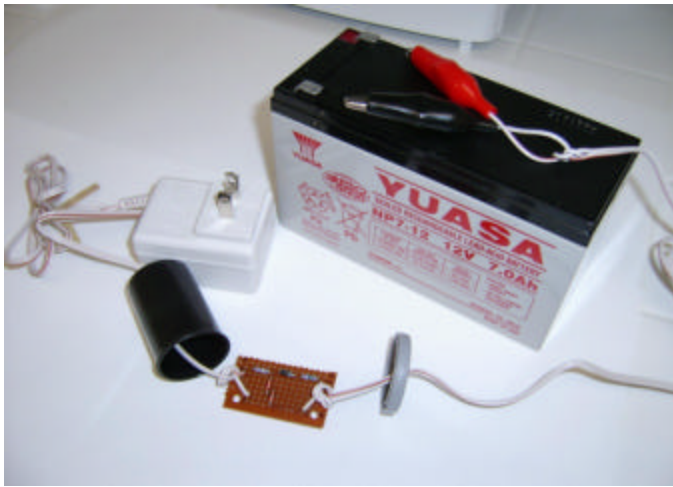
Andy's, W4ULD , Float Charger for Gel Cells. Built by WA0ZGL . Added 35mm plastic can as the circuit board housing.
